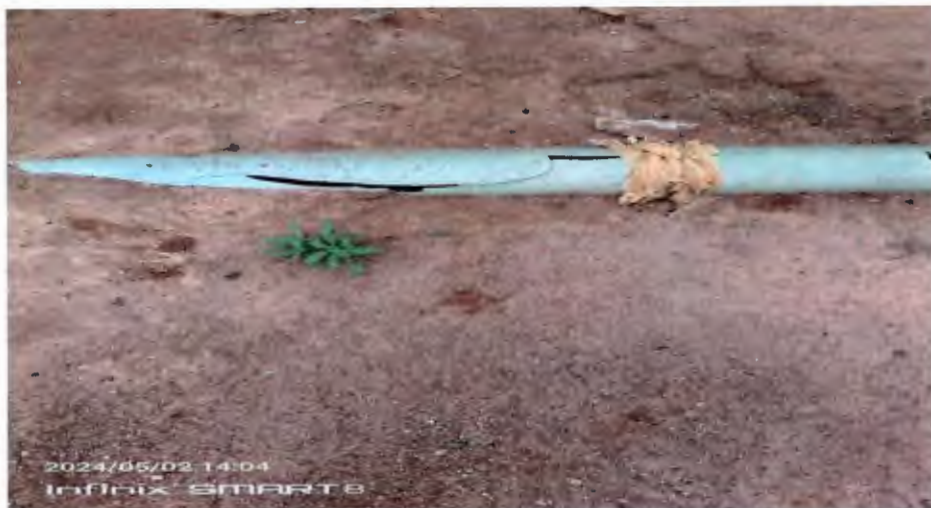
Bargblor, Grand Gedeh County Staff Housing Unit Damage sewage pipe
